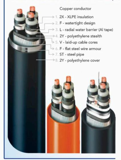
The advantages of pipe tye cables and XLPE cables are combined. The cable has been developed especially for use in urban cable networks for retrofitting and new installation. Major design details have been determined to take account of the use of existing cable pipe lines. This cables concept allows the cheap reconstruction of old pipe type cable circuits and the economical and safe installation of new cable connections in crowded city areas.
