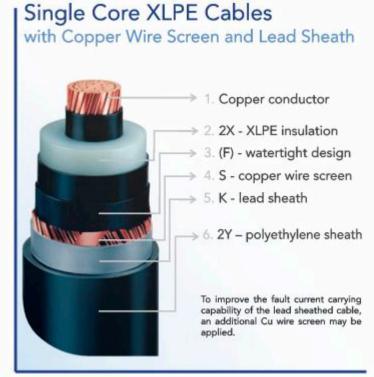
These cables can be supplied in the standard design, i.e. with insulation thickness as used already for several decades.
